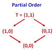
Meet Operator: Elementwise-min
